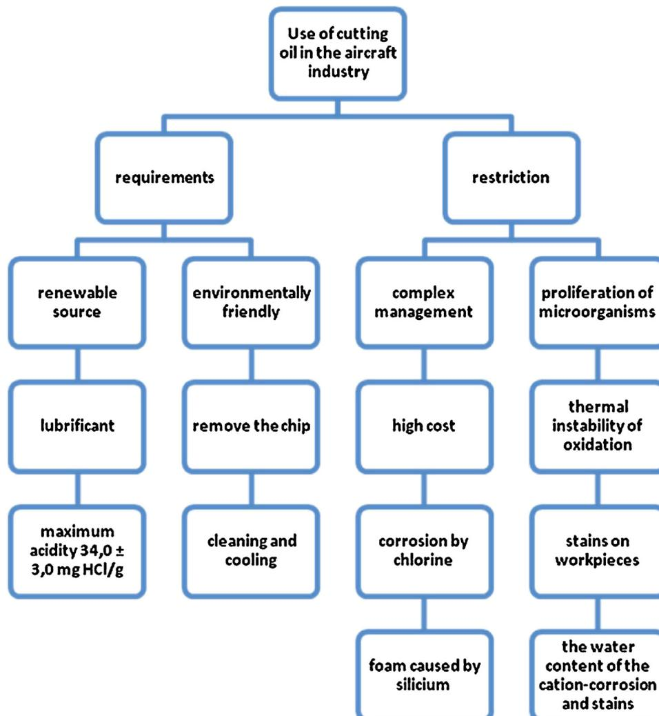
Fig. 1. Requirements and restrictions for the use of cutting fluid in the aeronautical industry.
