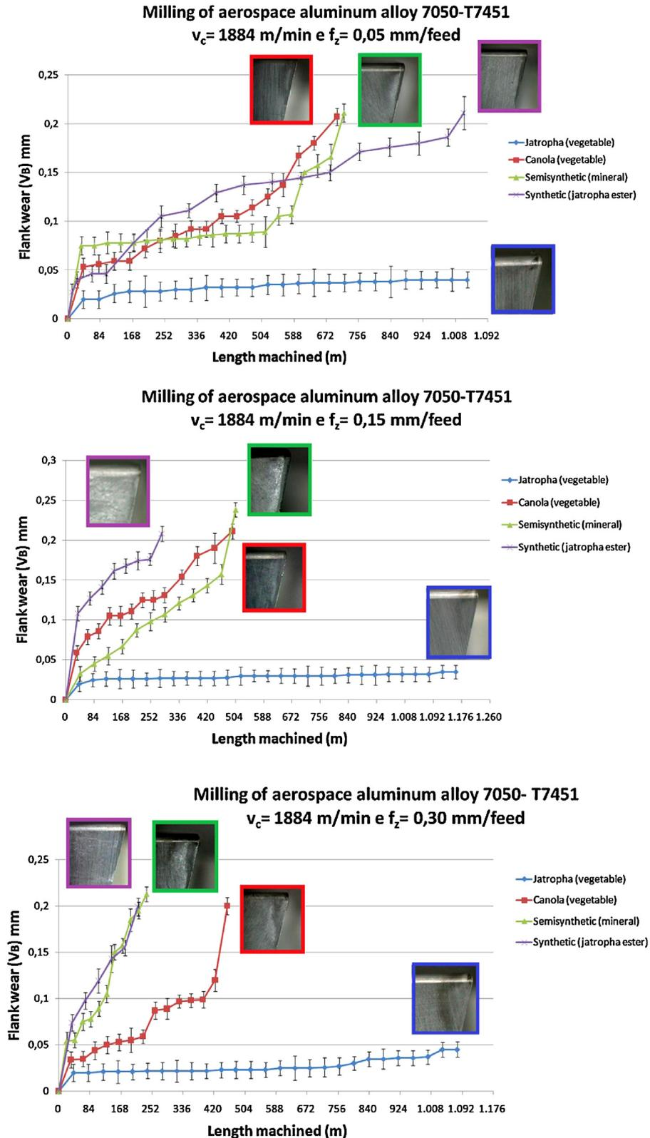
Fig. 3. Tool life with variation of cutting oil and feed rate  $[f_z]$  (mm/tooth).
