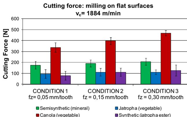
**Fig. 6.** Cutting force in the flat surfaces milling test.
