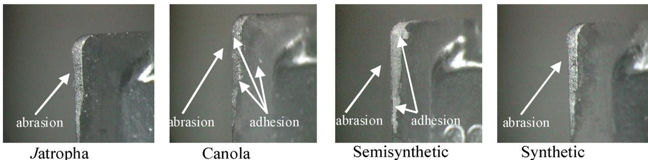
Fig. 4. Cutting tool surface wear outlet.
