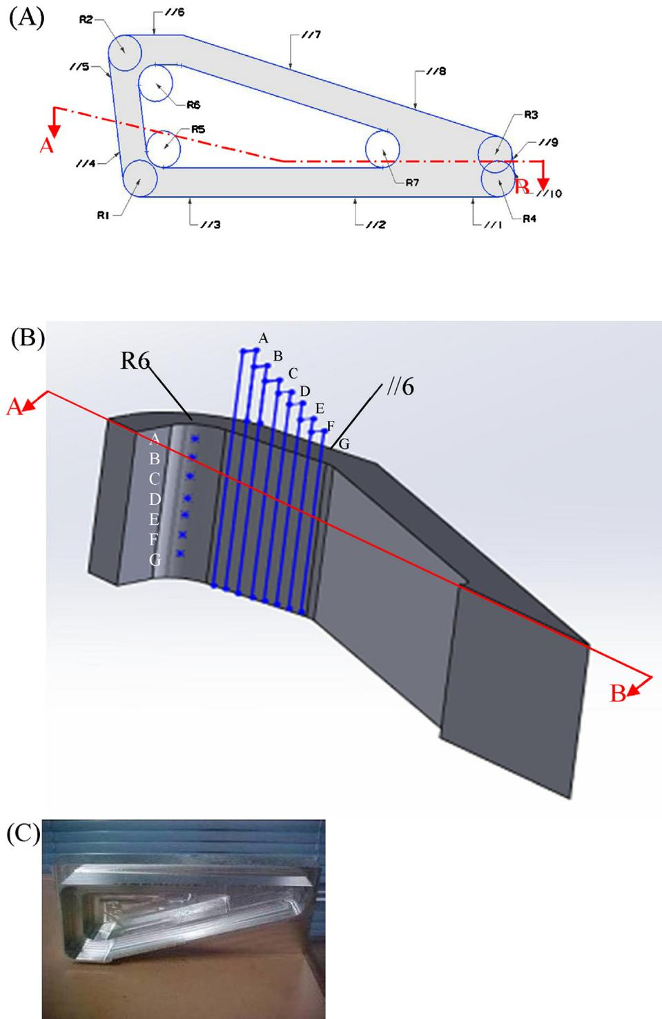
**Fig. 2.** Points and measurement locations shape errors in the model part. (A) Measurement points of shape errors on the model part and cut AB. (B) Cut AB: 7 measurement positions for mean determination, reference value for evaluation of shape errors. (C) Manufactured model part.
