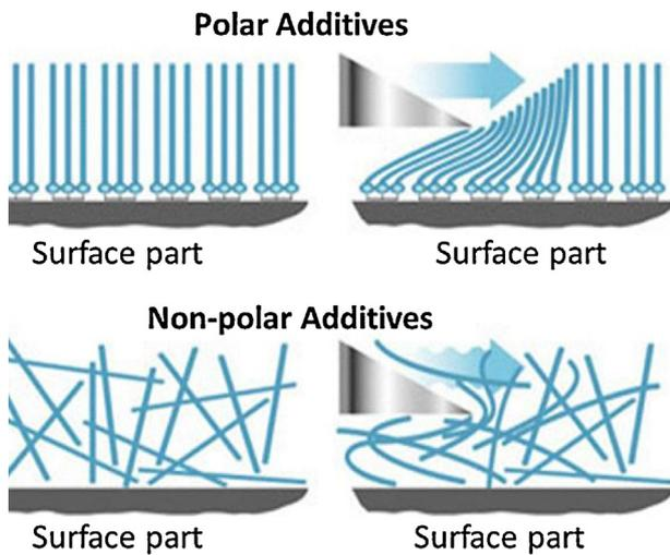
Fig. 8. Alignment scheme of mineral and vegetable oil molecules [43].
