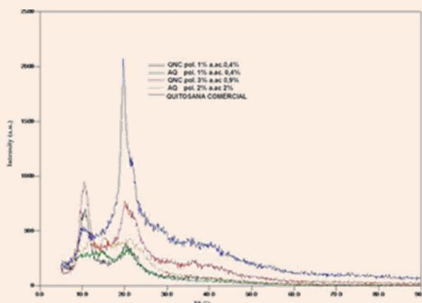
**Figure 7:** XRD pattern of the precursor chitosan acetate AQ (A) 1:0.4 and (D) 2:2% polymer concentration and acid concentration and the QNC (AI) 1:0.4 and (C-III) 3:0.9% polymer concentration and acetic acid concentration.
