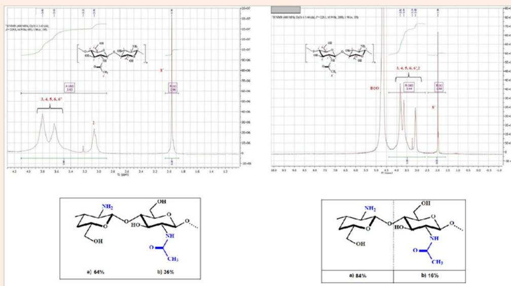
**Figure 8A & 8B:** H1 NMR Spectrum AQ and QNC in D2 O / HCl in a concentration of 5 mg / ml. The hydrogens are represented by numbers according to the carbon position which they are attached to deacetylated and acetylated monomer monomers. Often repetitive units occur in ethyl Chitosan, in percentage terms: (a) acetylated units; (B) deacetylated units.
