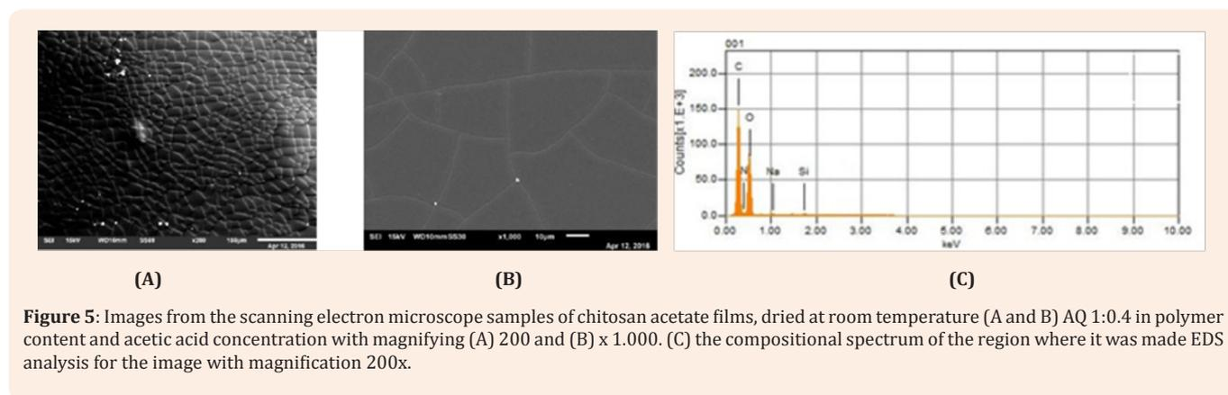
**Figure 5:** Images from the scanning electron microscope samples of chitosan acetate films, dried at room temperature (A and B) AQ 1:0.4 in polymer content and acetic acid concentration with magnifying (A) 200 and (B) x 1.000. (C) the compositional spectrum of the region where it was made EDS analysis for the image with magnification 200x.
