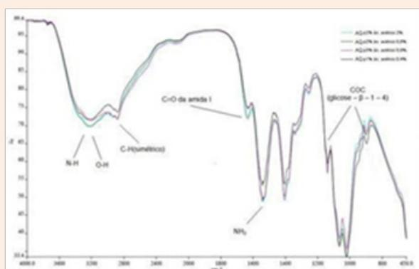
Figure 3: IR spectrum of chitosan in different concentrations.
